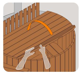
**2)** Flip the first section of the cover onto the adjacent one to facilitate the next step.
